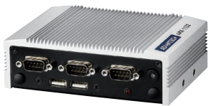
ARK-1122C-S6A1E •Intel Atom N2600 1.6GHz w/4COM+4USB+LAN
